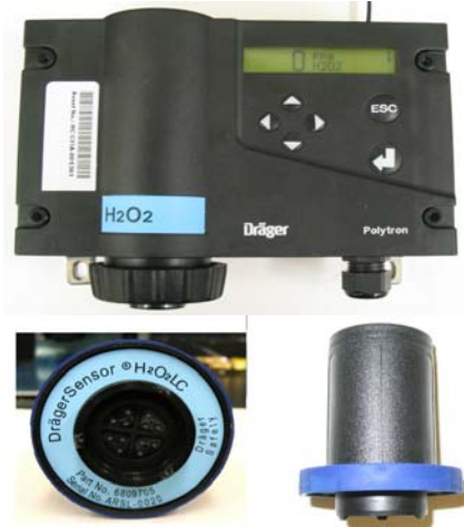
Fig. 3: Dräger Polytron 2 transmitter and H 2 O 2 electrochemical sensors. A high concentration sensor (0-7000ppm) connected to the transmitter was set up in the lab to monitor real-time VHP concentration
