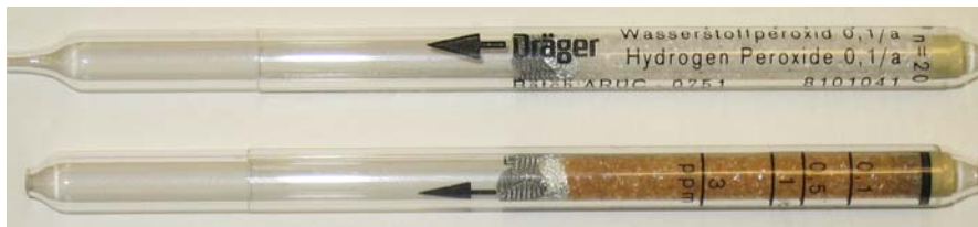
Fig.7: Dräger gas detection tubes for H 2 O 2 : Capable of determining VHP concentration between 0.1-3 ppm (semi quantitative). White crystals in the tube become brownish upon reaction with H 2 O 2 . After overnight ventilation, the lab read 0.3ppm residual VHP concentration, below the personal exposure level. Air samples in the surrounding areas of the lab tested negative for VHP during & after the biodecontamination process indicating the absence of VHP leak out of the lab.
