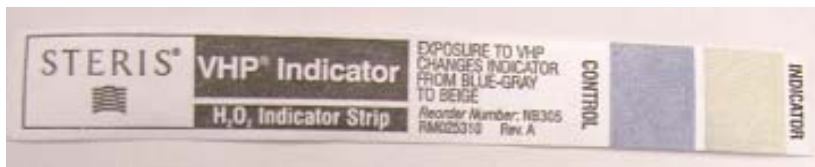
Fig.6: Chemical Indicator: Upon VHP exposure the blue colored indicator becomes beige. All 45 CIs changed color indicating that the VHP reached virtually everywhere in the lab.
